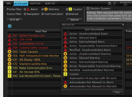
By clicking on the [icon] in the ACTIVE ALERT page, the list of icons used in the Alert Management System and their descriptions can be shown as a pop-up window.
