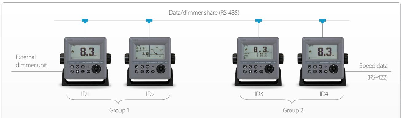
In this sample, the display with ID4 receives data (RS-422) from signal distributor and outputs vessel speed data (RS-485) to all connected display. Dimmer share has been separated in two groups, whereas group 1 can be operated by external dimmer and group 2 is linked pressing the button on the display.
