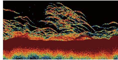
The high level of detail available with TruEcho CHIRP™ technology helps to distinguish fish schools, even when close to the sea bed.
