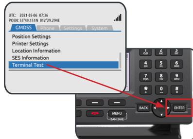
Use the 4-way navigation key to scroll all the way to the bottom to Terminal Test.
