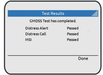
This screen shows that all tests were passed, and the terminal is working as expected.
