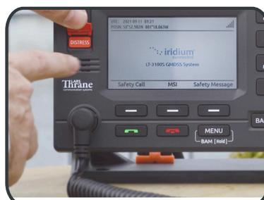
Lift the lid to the DISTRESS button and push the button for a minimum of three seconds.
