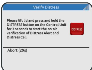
Press the DISTRESS button on the LT-3100S Control Unit to activate the Terminal Test.
