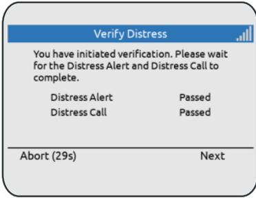
Each function will show "In Progress" until the test is complete.
