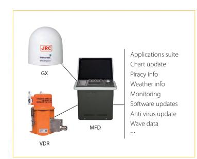
Dedicated high speed communications together with JRC newest generation onboard navigation equipment provides for seamless integration of support and applications, superfast and anywhere between 70 degrees North and South. Functions for captain and officers are directly accessible from our Multi Function Display (MFD).
