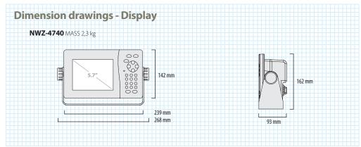
cutout for panel mount height 116,6 mm, width 220 mm, depth 180 mm
