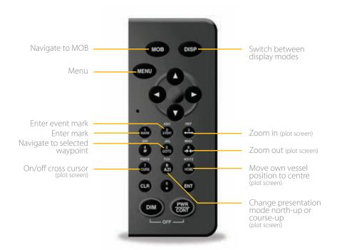
The keys are also backlit, making it easy to operate in low-light settings on the bridge.
