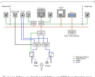
Dual non-follow-up direct / and follow-up CAN bus steering gear control system for a vessel with single rudder
