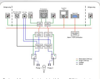
Dual non-follow-up direct / and dual follow-up CAN bus steering gear control system for a vessel with single rudder
