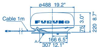
24" Radome Radar Sensor DRS4DNXT 7.3kg 16.1 lb
